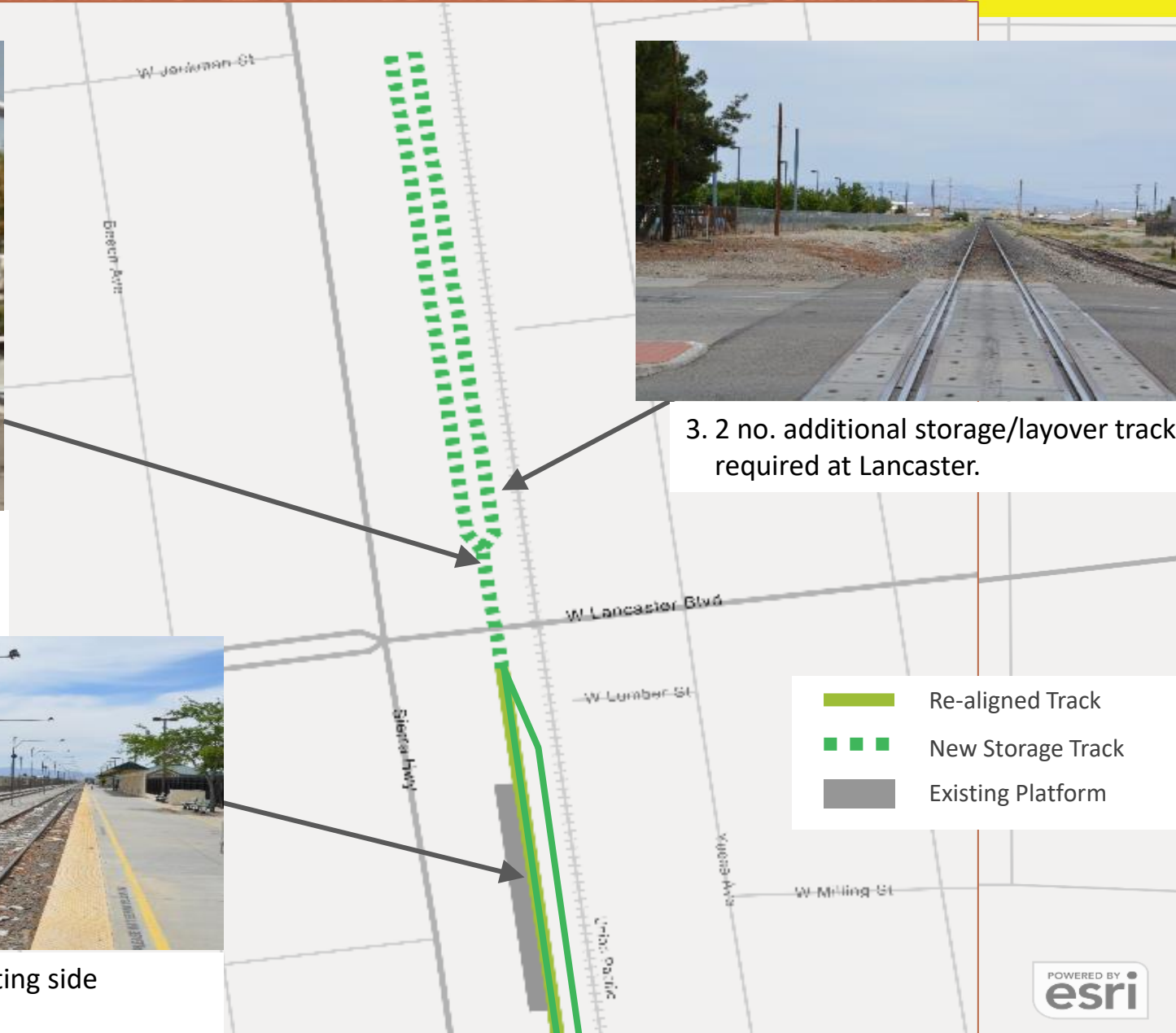
2. Modifications required at existing Lancaster Blvd grade crossing to allow trains to move to storage/layover tracks
