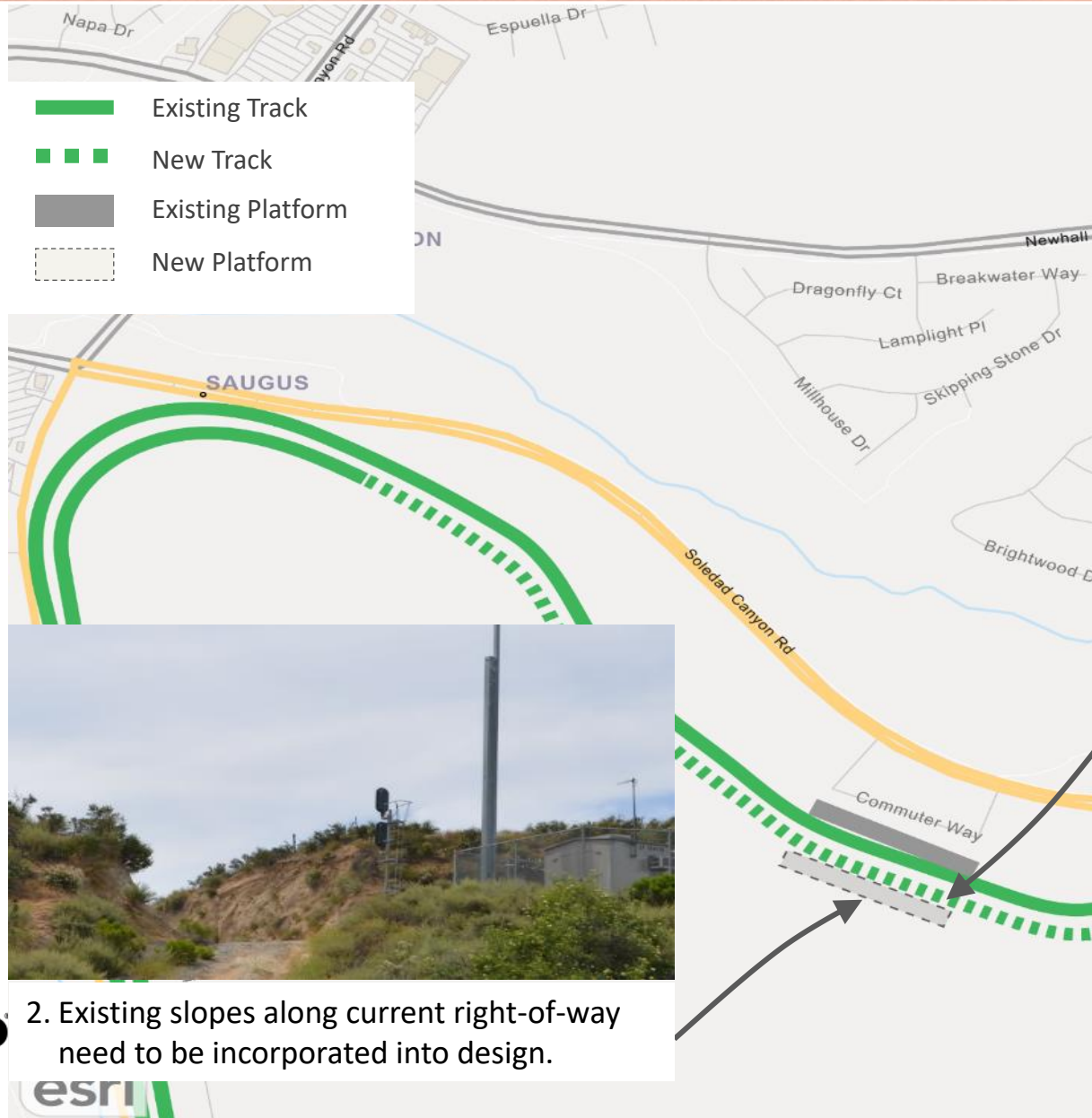
1. Second track and new side platform at Santa Clarita Station to be designed.
