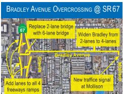
Bradley Avenue will be improved from east of SR-67 for a distance of 0.75 miles. The existing two lane Bradley Avenue bridge over SR-67 will be replaced to add turn lanes, bike lanes and sidewalks.
